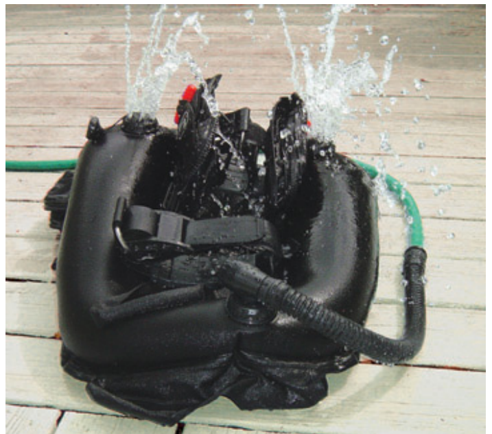
BC being flushed out using the standard garden hose connector
